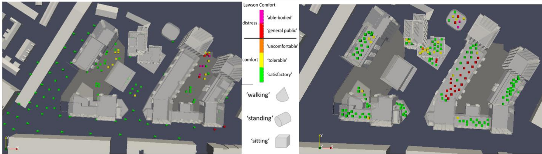
Figure 16.6: Lawson Comfort Criteria at Ground Level (left) and Terraces (right) without Wind Mitigation
